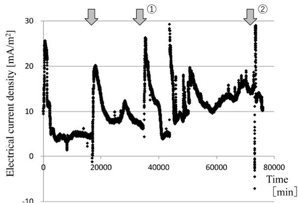
Fig. 3. Changes in current during batch operation of the methanogen cathode MFC. Arrow showed sampling time for analysis of water quality in the reactor. ①, ② showed the time for electrochemical analysis. ① showed 36000 times. ② showed 72000 times.
