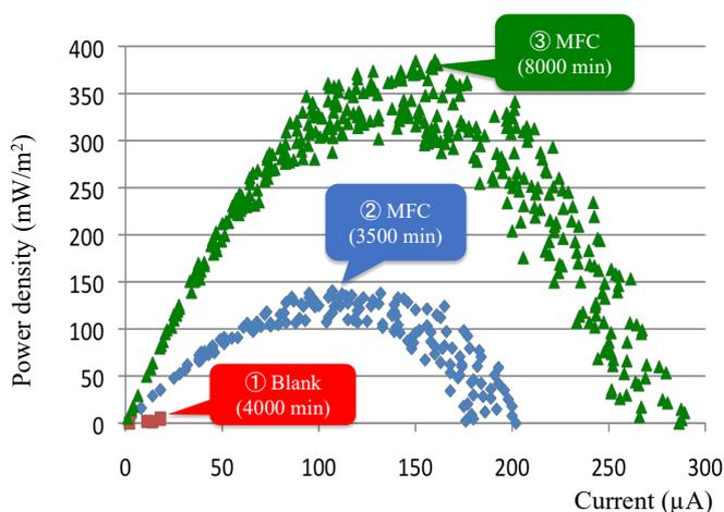
Fig. 7. Power density during continuous operation of the methanogen cathode MFC and the control cathode MFC (without methanogens).
