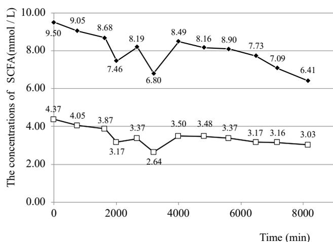
Fig. 8. SCFA concentrations in the anode bottle during continuous operation of the methanogen cathode MFC. Black rhombus showed the propionic acid concentration, and white square showed the acetic acid concentration.
