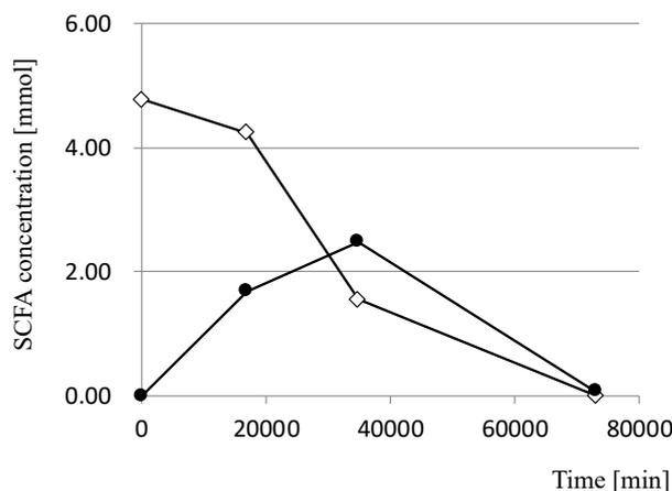
Fig. 4. SCFA concentrations in the anode bottle during batch operation of the methanogen cathode MFC. White rhombus showed the propionic acid concentration, black circle showed the acetic acid concentration.
