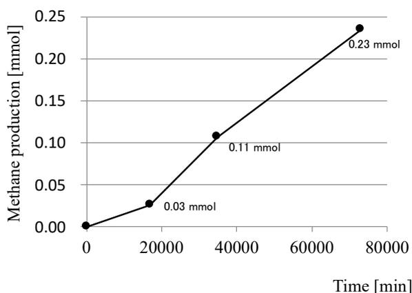
Fig. 5. Methane production in the cathode bottle during batch operation of the methanogen cathode MFC.
