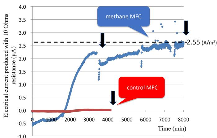
Fig. 6. Changes in current during continuous operation of the methanogen cathode MFC and the control cathode MFC (without methanogens).
