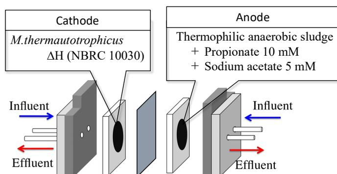
Fig. 2. Diagram of continuous operation of the methanogen cathode MFC.
