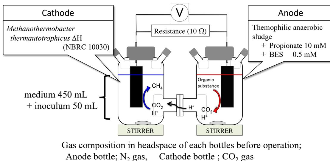
Fig. 1. Diagram of batch operation of the methanogen cathode microbial fuel cell (MFC).
